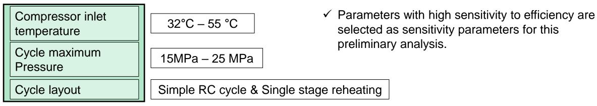
• Fixed parameters of SCO<sub>2</sub> cycle for 470MWt iPWR
