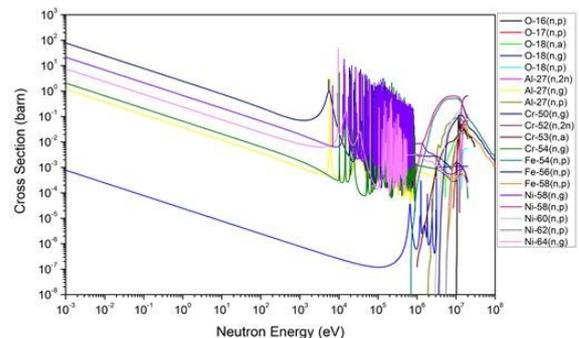
Fig. 1. Neutron cross section of the nuclides of Al<sub>2</sub>O<sub>3</sub>/ SS316L
