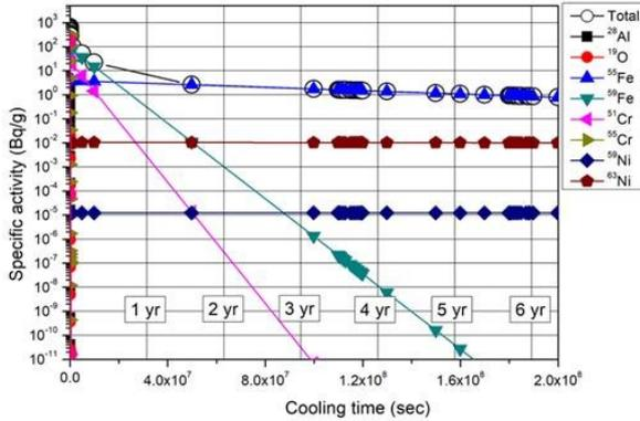
Fig.2. Specific activity of the Al<sub>2</sub>O<sub>3</sub>/ SS316L depending on the cooling time after the neutron irradiation of 3,000 sec
