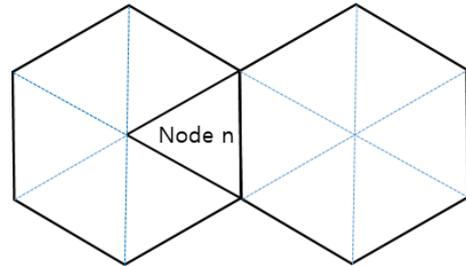
Fig. 1. Two adjacent hexagonal fuel blocks divided into trigonal nodes
