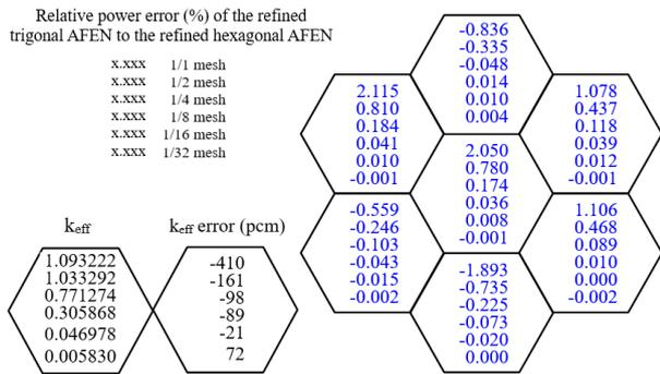
Fig. 4. Results of the MHTGR-350 benchmark problem with mesh refinement (1/12 core).
