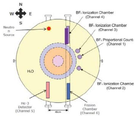
Fig2. Location of the detector in AGN-201K
