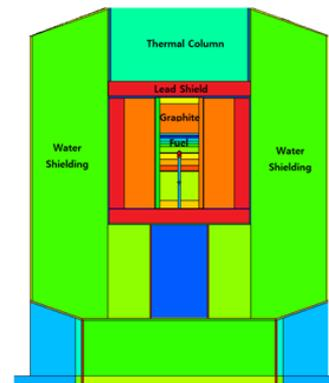
Fig. 1. Schematic diagram of AGN-201K
