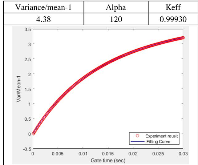
The AGN-201K operates with 4 control rods, and the criticality in all rod out state was 0.96202 when calculated using the MCNP6 code. The experiment was carried out using a data measurement device with a minimum gate time of 10 μsec (KHNP), and the processing was performed using the Moving Bunching Technique. In this study, noise analysis was performed from the critical condition to the deepest subcritical state, 0.96202, and the results were compared. This is shown in Figure 3 and Table 8.
