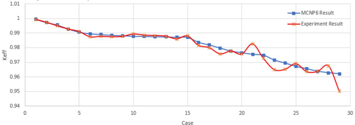
Fig3. Criticality curve of Feynman-alpha experiment result and MCNP6 code results
