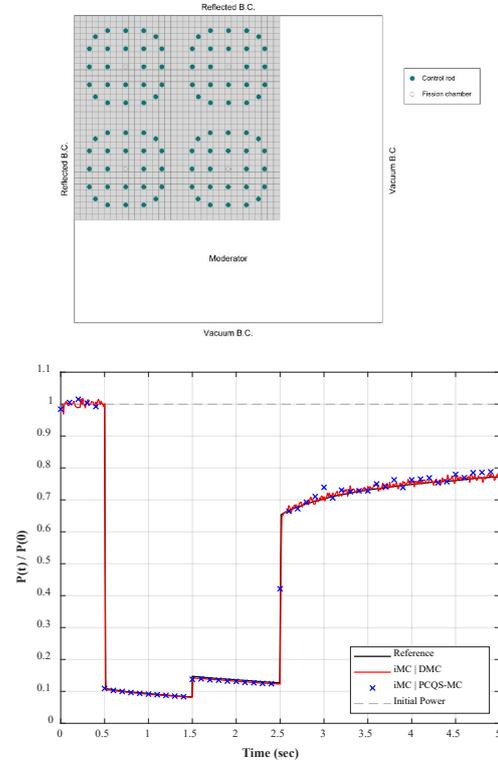
Figure 1. C5G7-TD problem geometry (top) and analysis results for C5G7-TD0-5 (bottom)
