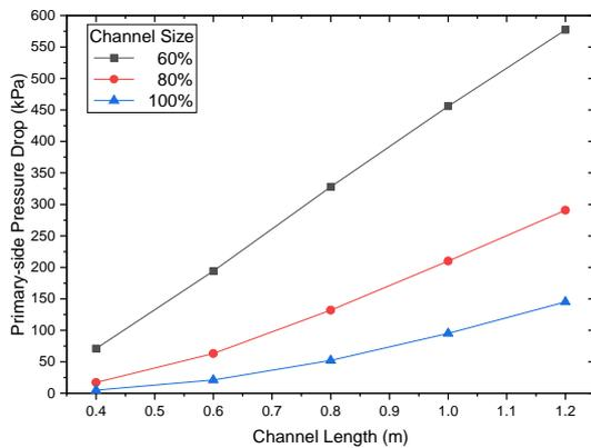
Fig. 3 Primary-side pressure drop
