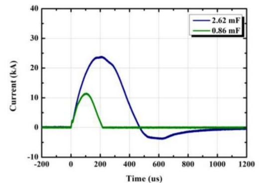
Fig. 6. Current waveforms for different capacitance values
