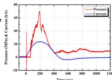
Fig. 5. Pressure and current waveform
