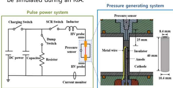
Fig. 2. Schematic of plasma-based RIA simulator
