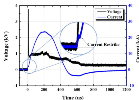
Fig. 4. Voltage and current waveforms measured at the load
