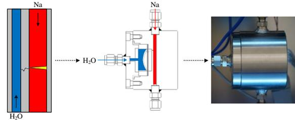
Fig. 5. Test section modeling and design
