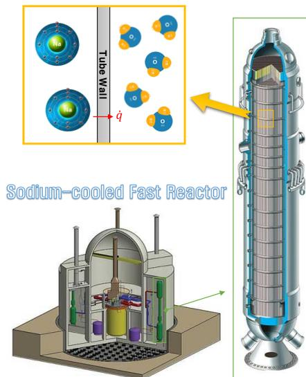
Fig. 1. Typical Steam Generator used in the SFR
