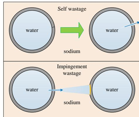
Fig. 2. Schematic Drawing of wastage phenomena
