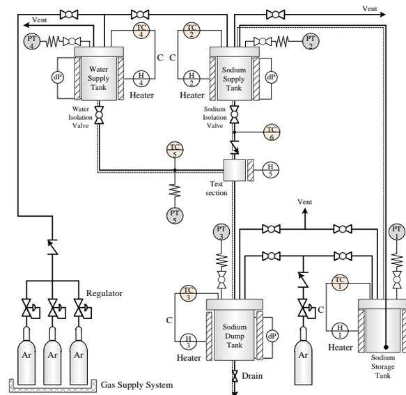
Fig. 6. P&ID of the CATS-S (Compact Accident Tolerance Steam Generator – SWR)
