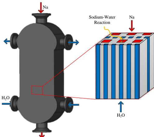
Fig. 4. Schematic of the PCSG and cross-sectional area
