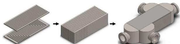
Fig.3. Fabrication procedure of the PCSG
