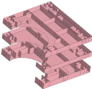
Fig. 1. The 3D FE model of auxiliary building
