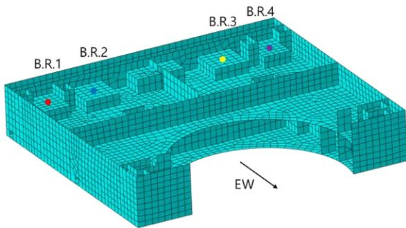
Fig. 4. The selected point of the auxiliary building
