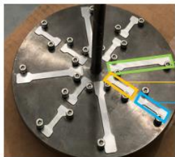
Fig. 3. Actual figure of specimens and specimen holder.
