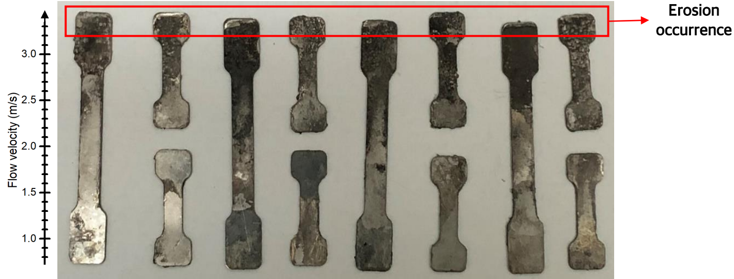
Specimens after cleaning using 150°C of glycerin
