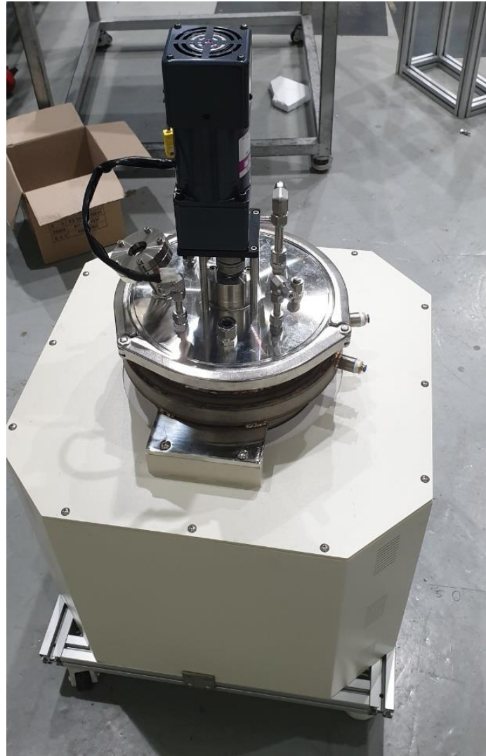
Actual figure of FAC experimental device and specimen holder
