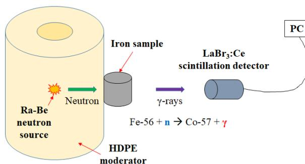
Fig. 2. Schematic diagram of prompt  $\gamma$ -ray measurement of iron sample using the LaBr<sub>3</sub>:Ce scintillation detector
