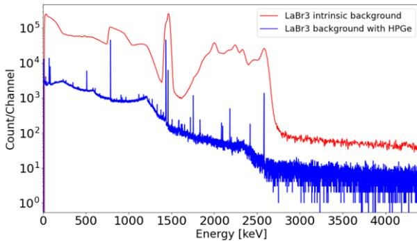
Fig. 3. The background spectra measured with the LaBr<sub>3</sub>:Ce scintillator and the HPGe detector. The red line is a self-radiation spectrum of LaBr<sub>3</sub>:Ce crystal, and the blue line is a spectrum from the HPGe detector.
