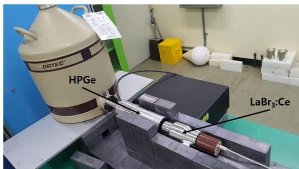
Fig. 1. Experimental setup of the LaBr<sub>3</sub>:Ce scintillator and the HPGe detector (later shielded totally with the lead blocks).
