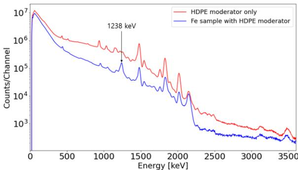
Fig. 4. Prompt  $\gamma$ -ray energy spectra of the iron sample measured by the LaBr<sub>3</sub>:Ce scintillation detector
