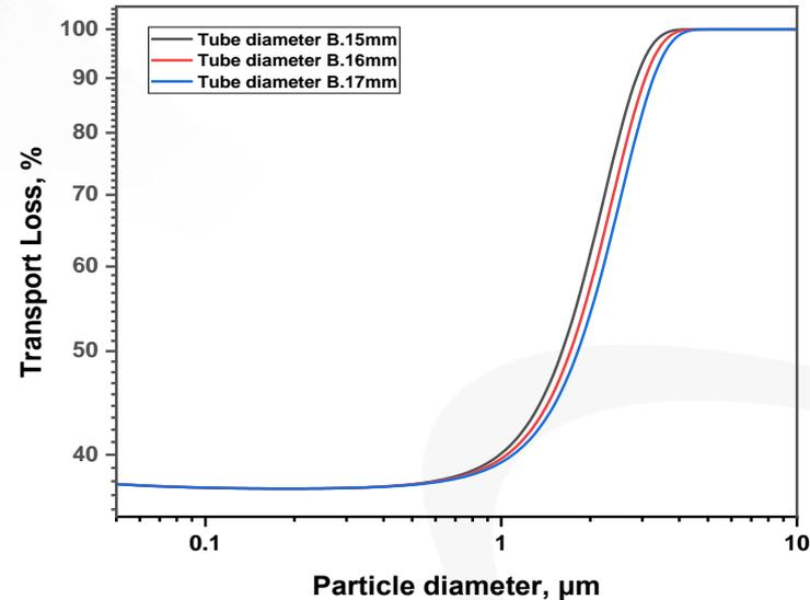
Fig. Transport loss with tube diameter B
