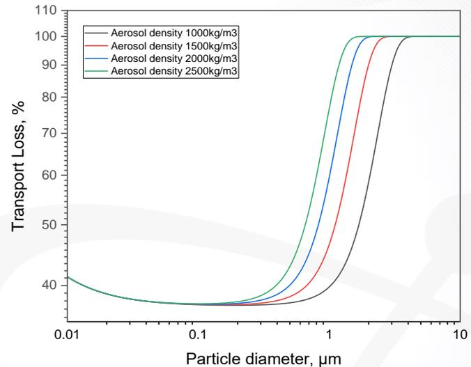
Fig. Particle loss with aerosol density.
