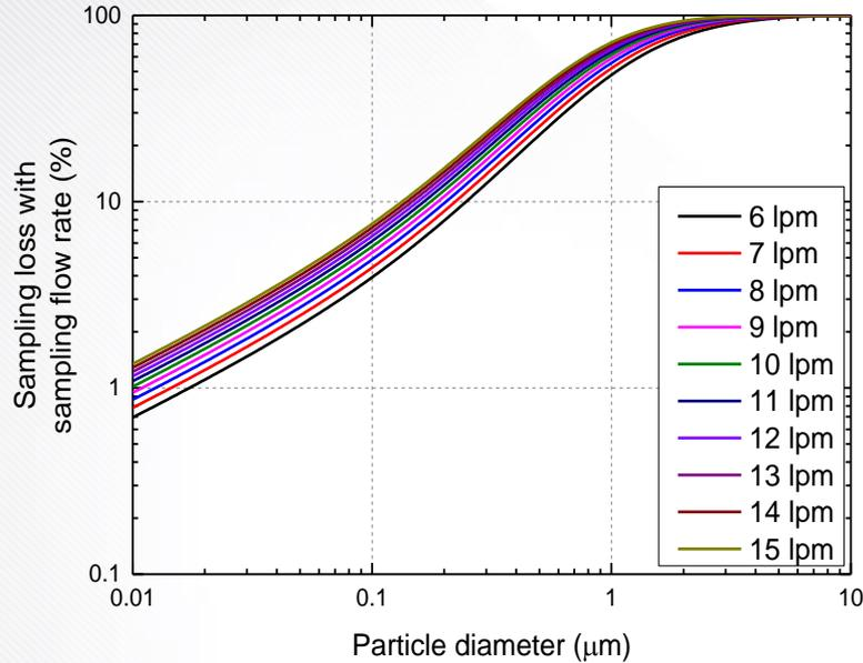
Fig. sampling loss with flow rate
