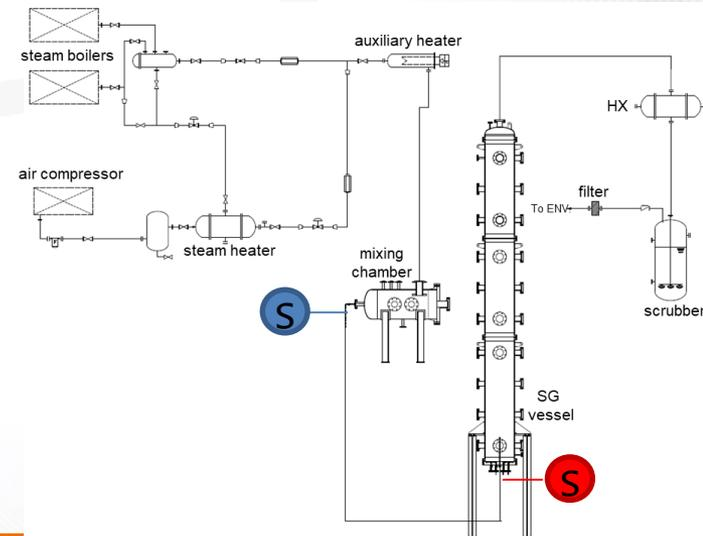
Fig. Schematics of SGTR exp. facility in KAERI
