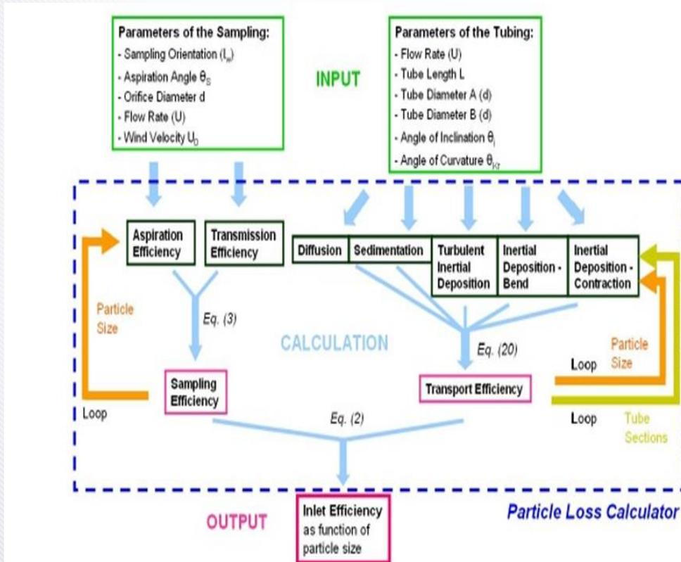
$$(\text{Inlet Efficiency}) = (\text{Sampling Efficiency}) \times (\text{Transport Efficiency})$$
