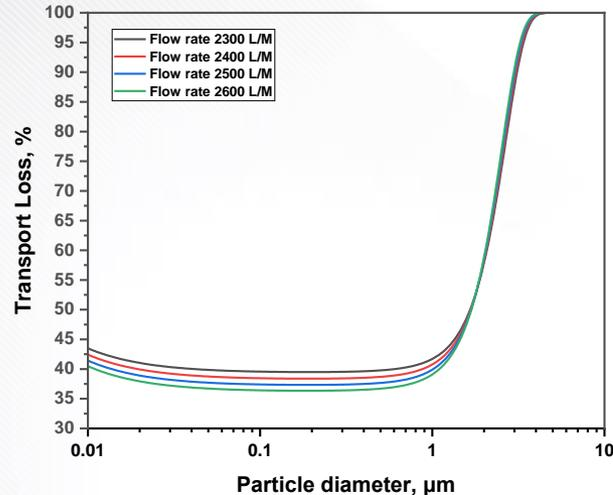
Fig. Transport loss with flow rate in pipe
