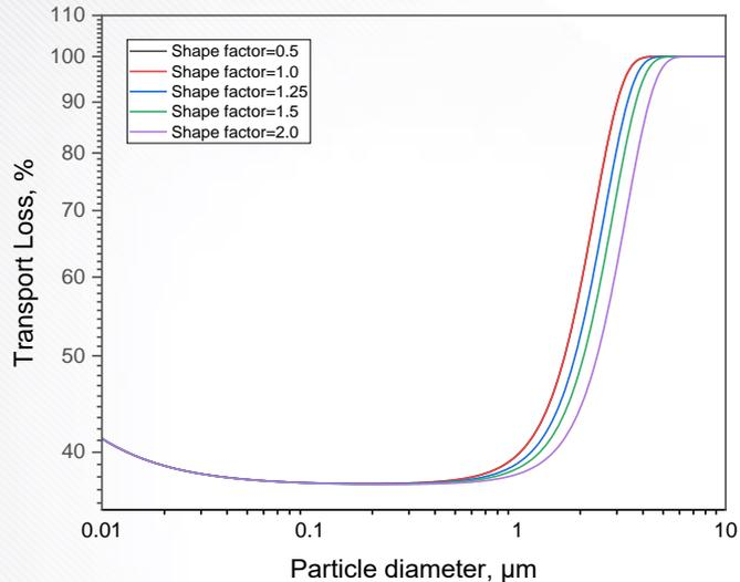
Fig. Particle loss with aerosol shape factor
