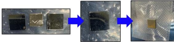
Fig. 3. Sample preparing process for positron annihilation lifetime spectroscopy (PALS). Glared blocks were advanced reduced-activation alloy (ARAA) samples, and light color is the positron source with a nickel foil
