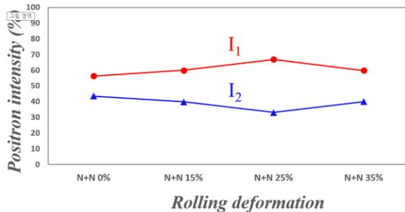
Fig. 5. Lifetime intensity of the samples in different rolling deformation
