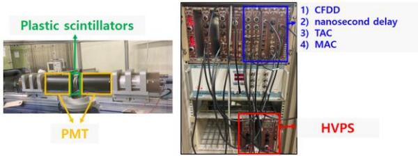
Fig. 2. Positron annihilation lifetime spectroscopy (PALS) system. PMT: photomultiplier tube HVPS: high voltage power supply, CFDD: constant fraction discriminator, TAC: time-to-amplitude converter, MCA: multi-channel analyzer.
