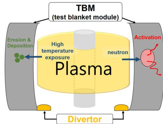
Fig. 1. The structure of the test blanket module (TBM) and divertor on the first wall of the international thermonuclear experimental reactor (ITER) and the effects of nuclear reactions
