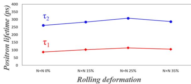
Fig. 4. Short and long lifetime of the samples in different rolling deformation.
