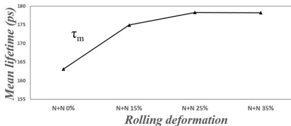
Fig. 6. Mean lifetime ( $\tau_m$ ) of the samples in different rolling deformation
