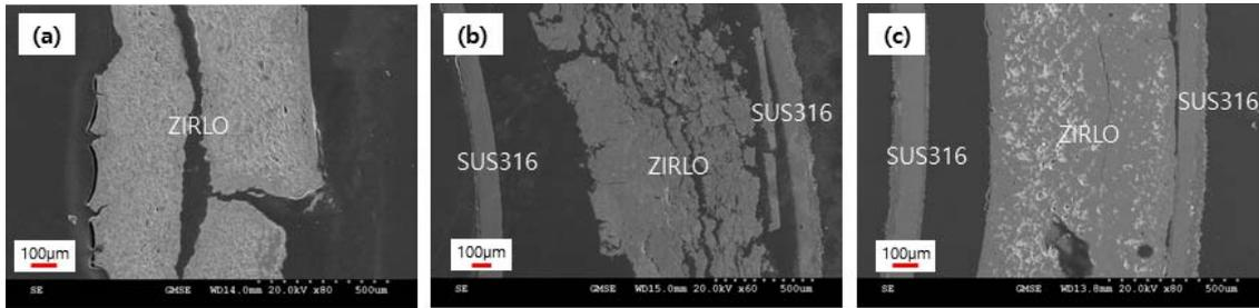
Fig. 4. SEM cross-sectional images of after 1200°C heat treatment: (a) ZIRLO; (b) 9.5Φ MWDC; (c) 9.4Φ MWDC
