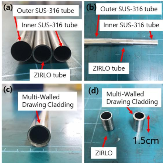
Fig. 2. Sample preparation process pictures: (a) Comparison picture of each tube diameter; (b) Tube assembly before drawing; (c) Photo of Multi-Walled Drawing Cladding (MWDC); (d) Samples cut for examination and heat treatment testing.
