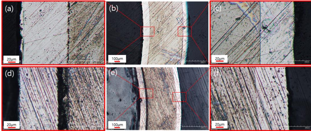
Fig. 3. Cross-sectional OM images (a) to (c) for 9.4Φ MWDC, and (d) to (f) for 9.5Φ MWDC, to analysis each specimen interface.
