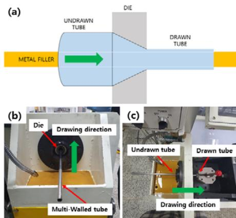
Fig. 1. Images of the drawing process (a) schematic diagram of the drawing and (b) a photograph of a sample placed into the machine, and (c) a photograph during drawing.
