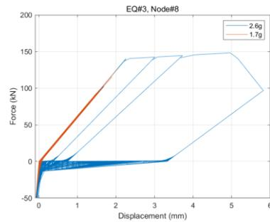
Fig. 8. Force-displacement of an anchor in z-dir.
