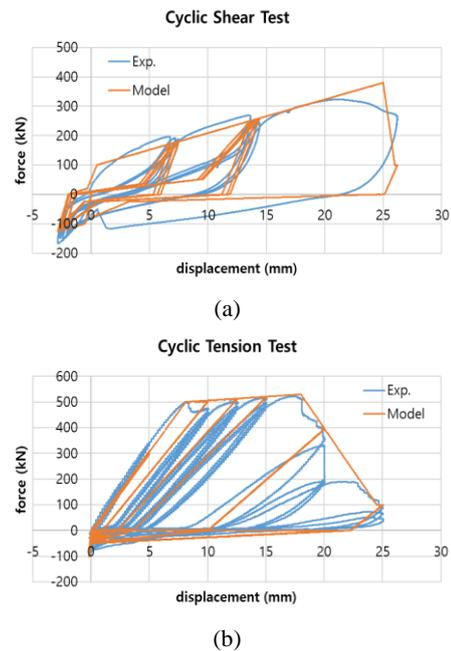
Fig. 2. Experimental results of anchor behavior : (a) cyclic shear test(x-y-dir.), (b) cyclic tension test(z-dir.)
