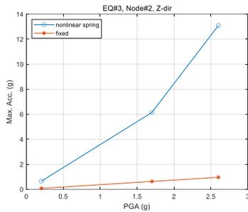
Fig. 10. Spectral acceleration of pump in z-dir. (node 2)
