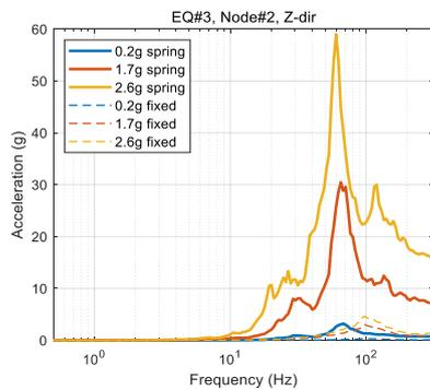
Fig. 10. Response spectrum of pump in z-dir. (node 2)
