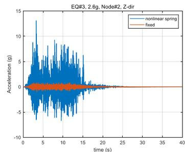
Fig. 9. Time-acceleration response of pump in z-dir. (node 2)
