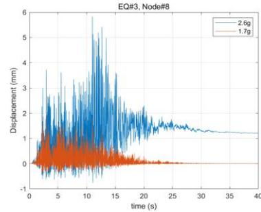
Fig. 7. Time-displacement response of an anchor in z-dir.
