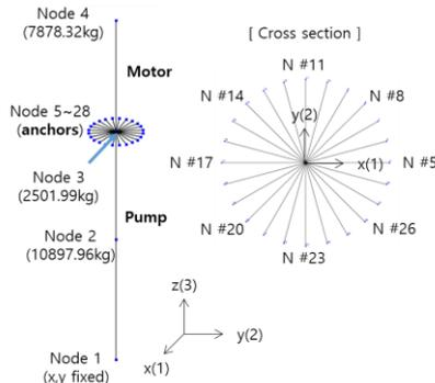
Fig. 5. Structural model of ESW pump
