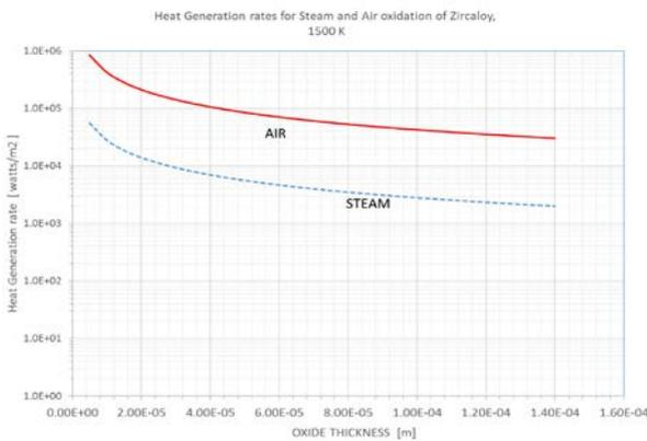
Fig. 5. Heat generation rates at one temperature and a range of oxide thicknesses.
