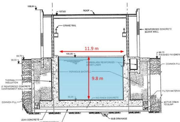
Fig. 2. Cross sections of the Spent Fuel Pool.
