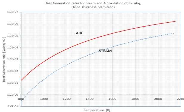
Fig. 4. Heat generation rates at a moderate oxide thickness of 50 microns.
