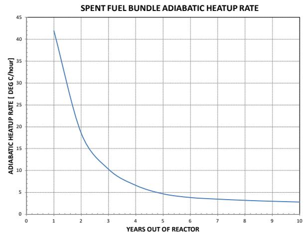
Fig. 3. Schematic Average fuel bundle adiabatic heatup rate
