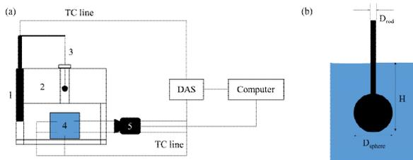
Fig. 1. (a) Diagram of the experiment system. (1 : pneumatic cylinder, 2 : furnace, 3 : support rod, 4 : water pool, 5 : high-speed camera) (b) Geometry of the specimen.
