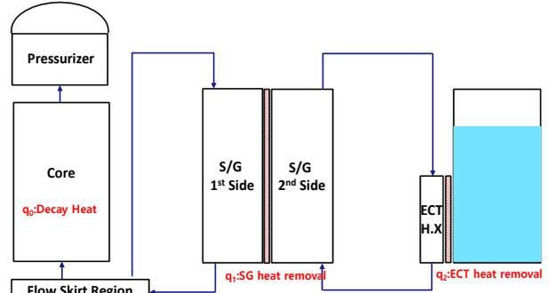
Figure 3. Schematic of the Energy Balance of SMART
