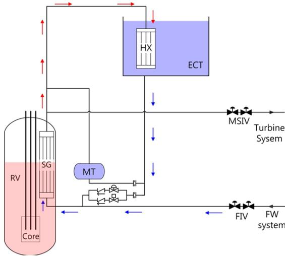
Figure 2. The Schematic of PRHRS
