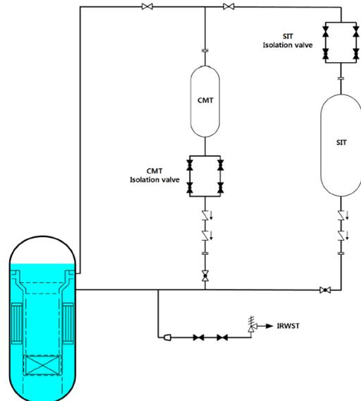
Figure 1. The Schematic of PSIS
