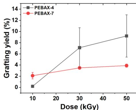
Fig. 1. Effect of absorbed dose on grafting yield of poly(AAc) grafted PEBA.
