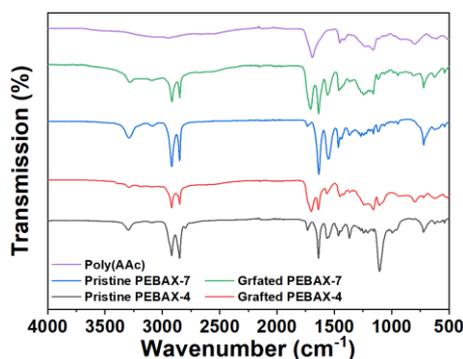
Fig. 2. FT-IR spectra of poly(AAc) grafted PEBA.
