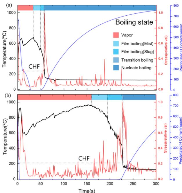
Fig.12. LOCA integral analysis of UCN 3&4. (a) Axial location 1.17m, (b) axial location 2.99m
