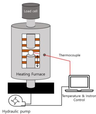
Fig.5. Ring compression test apparatus
