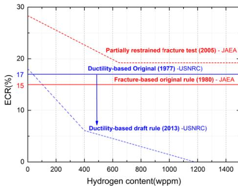
Fig.1. Ductility-based and Fracture-based criteria for high-burnup fuel
