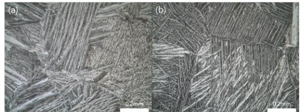
**Fig.9.** Microstructure of Prior-β phase layer. (a) 800°C quench, (b) 1200°C quench.
