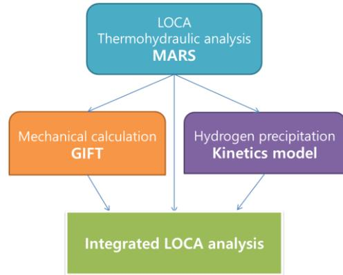
Fig.6. Schematic for Code-integrated LOCA analysis
