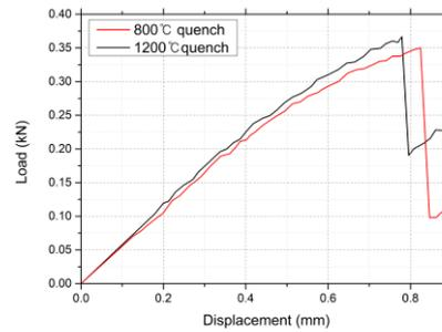
**Fig.10.** RCT results of ECR 17%, 1200°C quench and 800°C quench.
