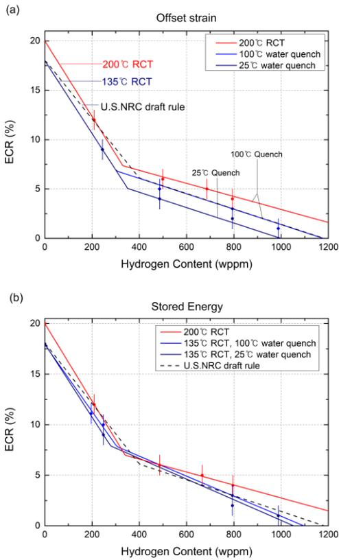
**Fig.7.** RCT results of Pre-hydrated and oxidized specimen at 135°C-100°C water quench, 135°C-25°C water quench, 200°C-100°C water quench. (a) Offset strain criteria, (b) stored energy criteria
