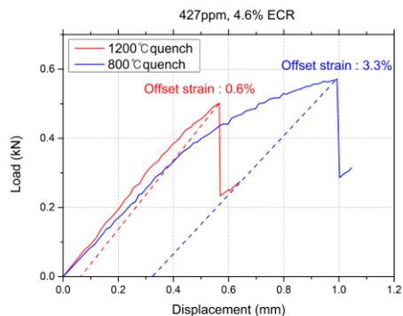
**Fig.11.** RCT results for 1200°C and 800°C quenched H 427wppm-ECR 4.6% specimen
