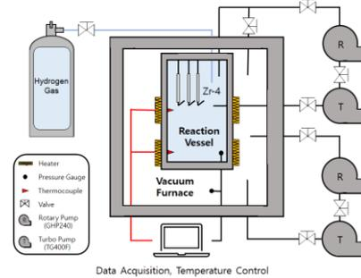
Fig.2. Gaseous hydrogen charging apparatus
