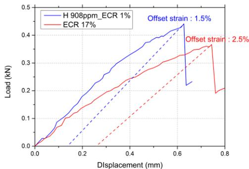
**Fig.8.** RCT result of H 0wppm, ECR 17% specimen and H 908wppm-ECR 1% specimen
