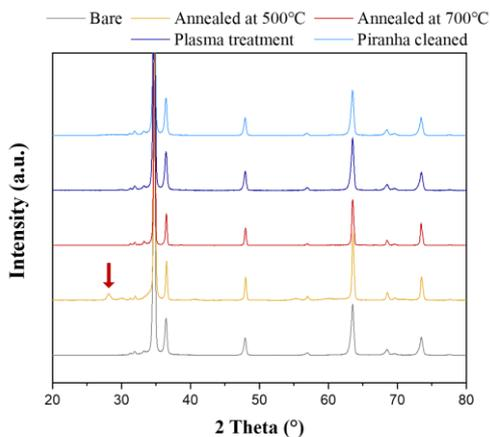
Figure 3. Representative XRD spectra according to surface treatment
