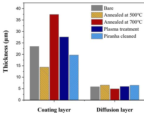
Figure 2. Thickness comparison in each specimen after vitrification
