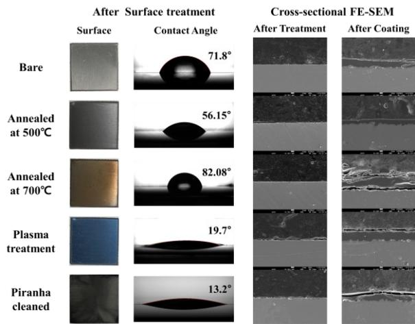
Figure 1. Case comparison after surface modification
