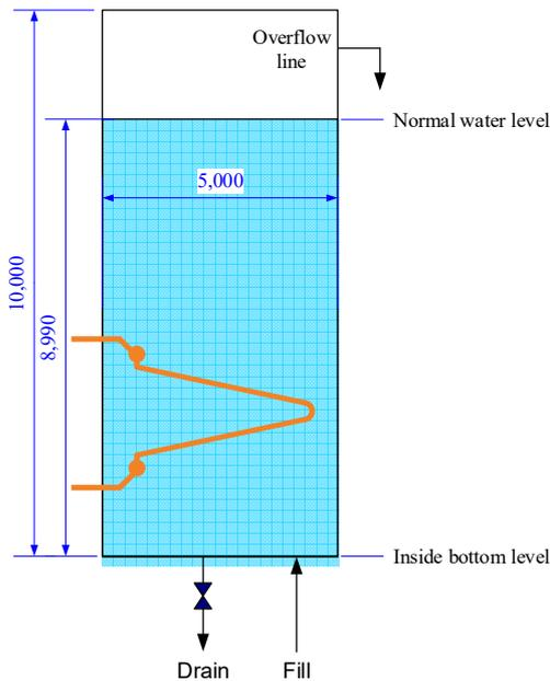
Fig. 3 Passive Condensation Cooling Tank (unit: mm)
