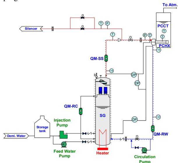
Fig. 1 Schematic diagram of LAPLACE test facility
