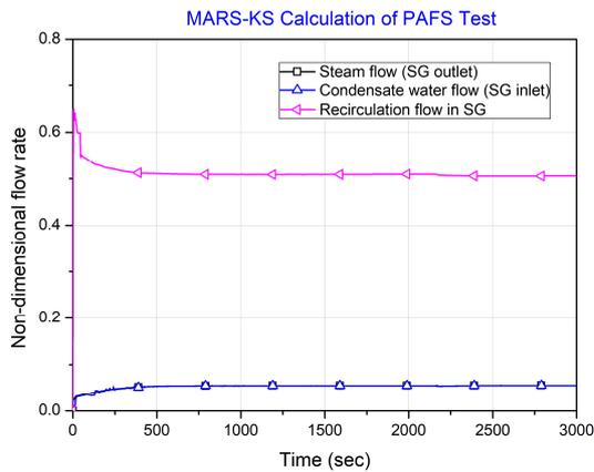
**Fig. 5 Natural convection flow in the MARS-KS calculation**
