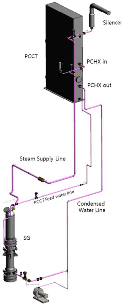
Fig. 2 Isometric view of the LAPLACE test facility
