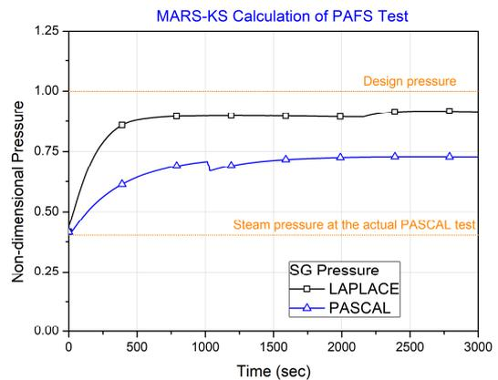
Fig. 4 Steam pressure in the MARS-KS calculation
