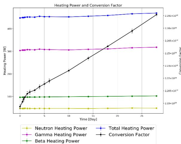
Fig. 2 Nuclear heating power with constant power
