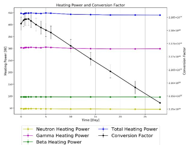
Fig. 3 Nuclear heating power with constant flux
