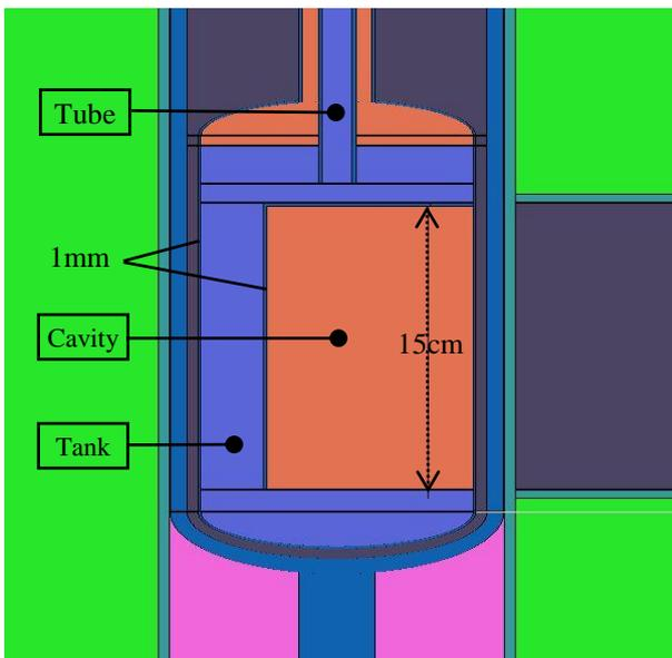
Fig. 1. The cross-sectional view of CNS moderator cell
