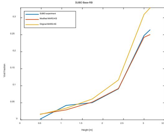
Fig. 8. Void fraction of SUBO experiments and MARS-KS prediction results – extreme case
