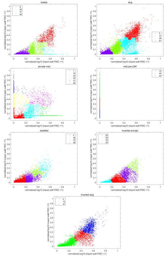
Fig. 4. Wall friction clustering results according to the flow regime [2]
