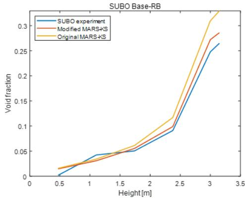
Fig. 5. Void fraction of SUBO experiments and MARS-KS prediction results
