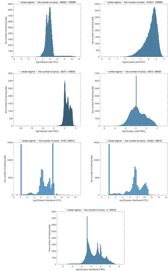
Fig. 1. Training data (a~g: coefficient of liquid wall HTC, vapor wall HTC, liquid wall FRIC, vapor wall FRIC, liquid interfacial HTC, vapor interfacial HTC, interfacial FRIC) [1]
