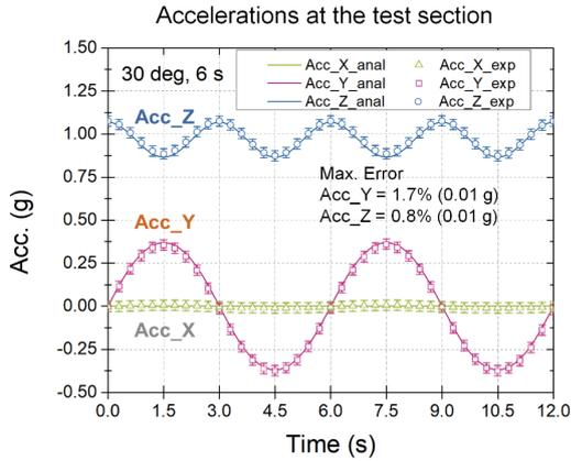
Fig. 2. Comparison result of acceleration at the test section under rolling condition (Experimental vs. analytic values)
