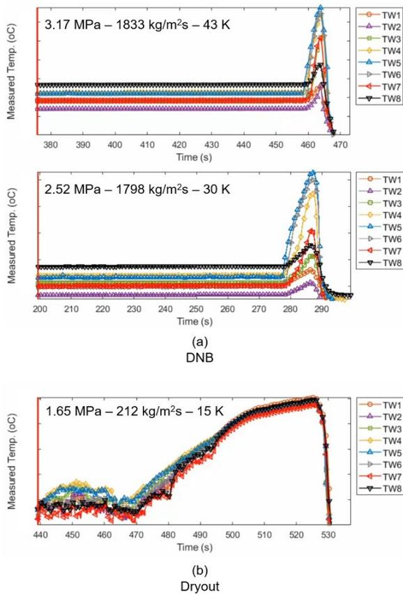
Fig. 4. Wall temperature response of heater rod for (a) DNB and (b) dryout under stationary vertical condition
