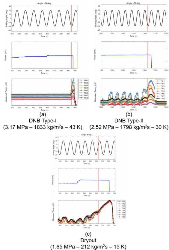
Fig. 5. Wall temperature response of heater rod for (a) DNB type-I (b) DNB type-II (c) dryout under rolling condition
