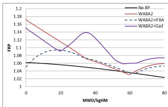
Fig. 7. Comparison of radial power peaking factor for WABA2, WABA2+IFBA and WABA2+Gad cases.
