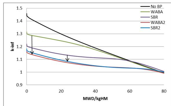
Fig. 3. Comparison of excess reactivity for WABA, SBR, WABA2 and SBR2 cases.
