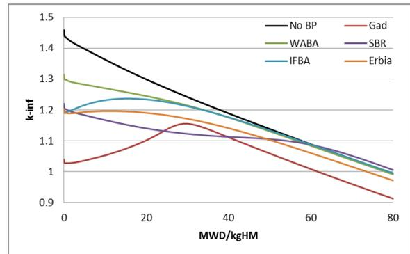
Fig. 2. Comparison of conventional BP types effect on excess reactivity.
