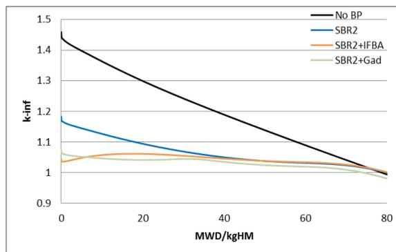
Fig. 6. Comparison of excess reactivity for SBR2, SBR2+IFBA and SBR2+Gad cases.
