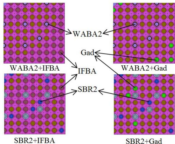
Fig. 4. 1/4 WH fuel assembly with different BP pins loading (WABA2+IFBA, WABA2+Gad, SBR2+IFBA & SBR2+Gad).
