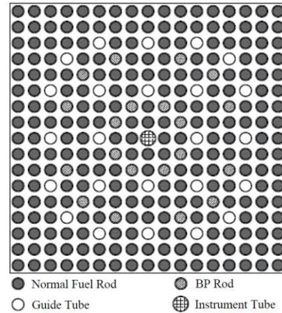
Fig. 1. Standard WH fuel assembly type.
