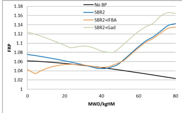
Fig. 8. Comparison of radial power peaking factor for SBR2, SBR2+IFBA and SBR2+Gad cases.
