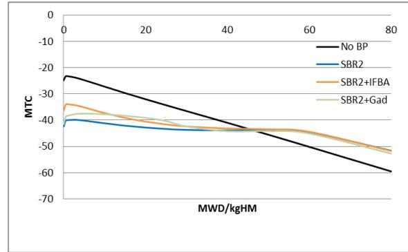
Fig. 10. Comparison of MTC for SBR2, SBR2+IFBA and SBR2+Gad cases.
