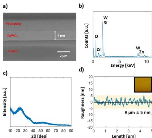
Fig. 2. a) Cross-sectional SEM images of the bare ZnWO<sub>4</sub> obtained by FIB , b) EDX spectrum of the bare ZnWO<sub>4</sub> film, c) XRD spectrum of the bare ZnWO<sub>4</sub> film, d) the surface morphology and roughness of the bare ZnWO<sub>4</sub> film by AFM analysis
