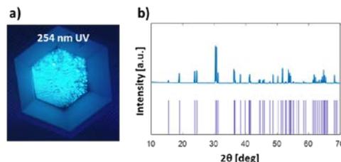
Fig. 1. a) ZnWO<sub>4</sub> powders irradiated by 254 nm UV, b) XRD spectrum of ZnWO<sub>4</sub> powders
