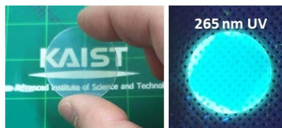
Fig. 4. Nano-grained thin-layer transparent ZnWO<sub>4</sub> scintillator film
