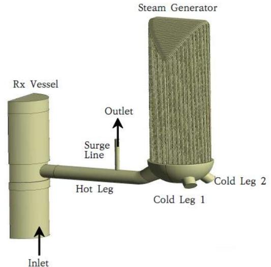
Fig. 3. Grid Model for Simulating Natural Circulation Flow in the Hot Leg and SG Inlet Plenum of OPR1000 [6]
