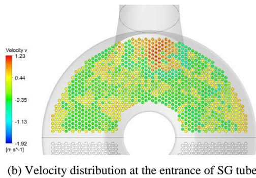
Fig. 4. CFD Results of Natural Circulation Flow in the Hot Leg and SG Inlet Plenum of the OPR1000
