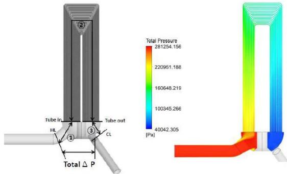
Fig. 2. Pressure Distribution by the CFD analysis using d Standard k-ε Turbulent Model
