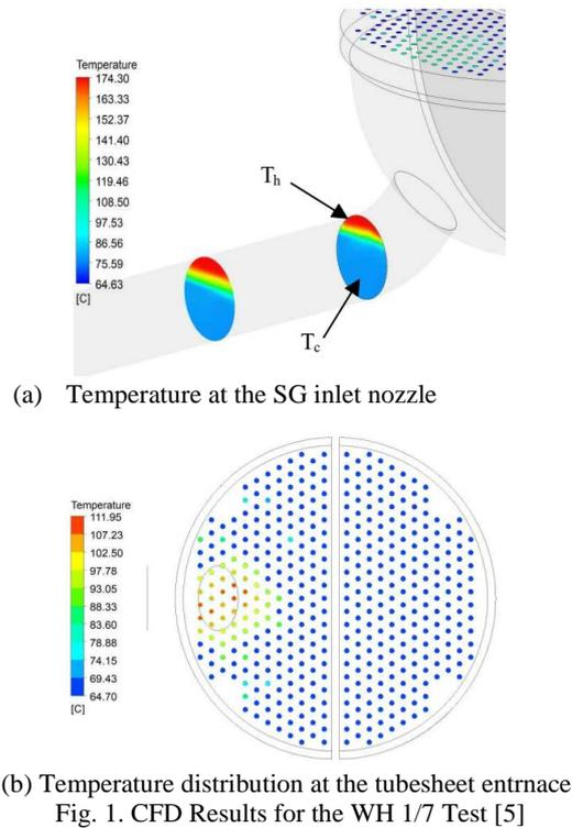
Fig. 1. CFD Results for the WH 1/7 Test [5]
