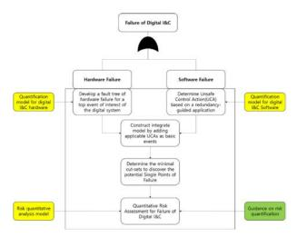
Fig. 2. The progress of failure analysis methodology for digital I&C systems.
