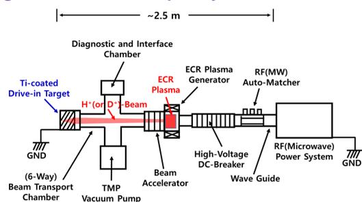
Fig. 1. Schematic structure of hydrogen ion beam test facility
