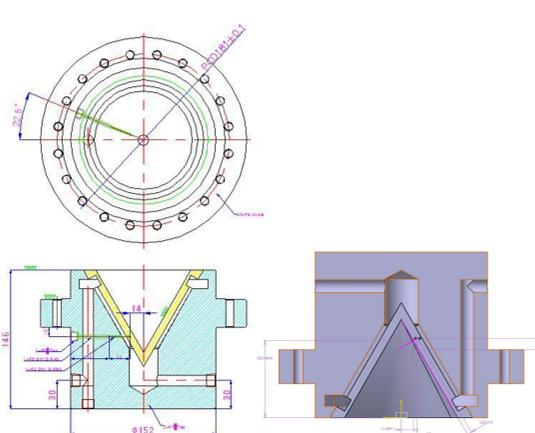
Fig. 4. Designed structures of water-cooled solid-target (including a beam target, a target supporter, and a thermocouple hole)
