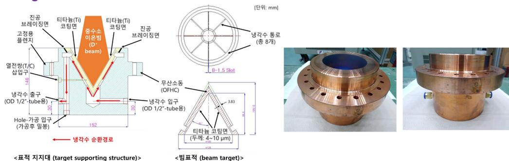
Fig. 6. structures of fabricated and assembled water-cooled solid-target
