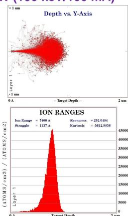
Fig. 3. Calculation results for injected depth of deuterium ion particles inside the titanium layer (by simulation of SRIM code)
