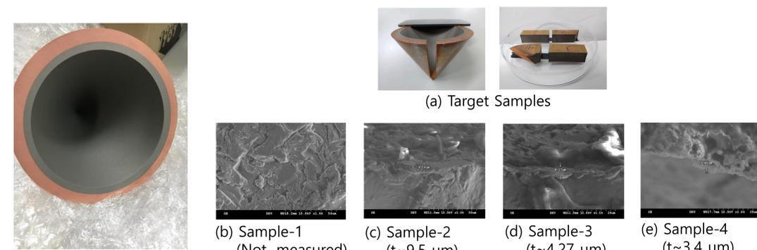
Fig. 7. A photo of titanium coated beam target
