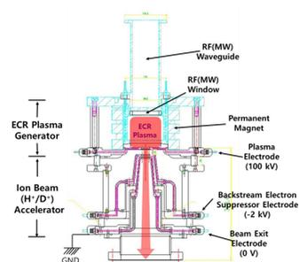
Fig. 2. Schematic structure of ECR ion source
