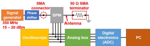
Fig. 1. Schematic diagram of the test setup
