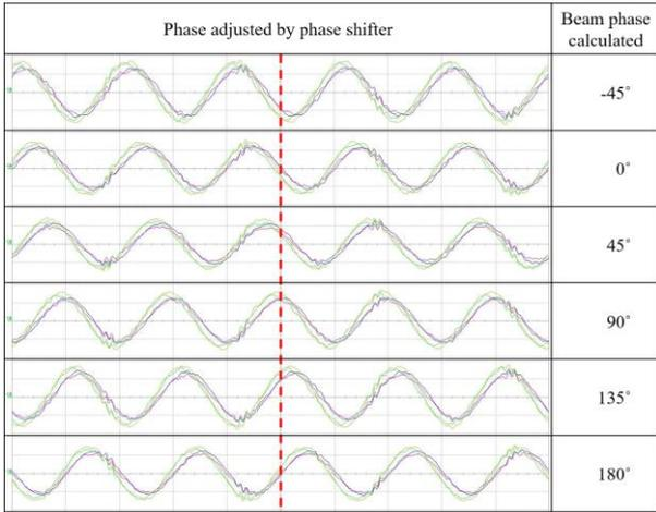
Fig. 5. Beam phase measurement by adjusting through the phase shifter.
