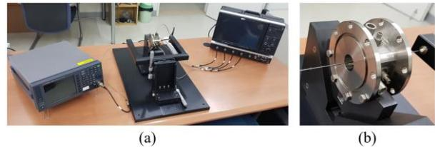
Fig. 2. BPM test stand: (a) total setup, (b) the BPM transducer and the antenna wire.
