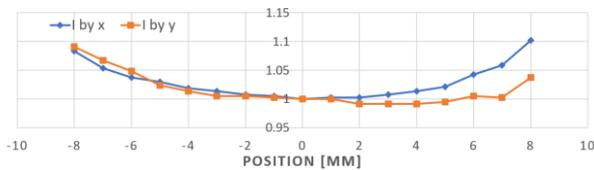
Fig. 6. The normalized beam current value by the position of the simulated beam (antenna wire)
