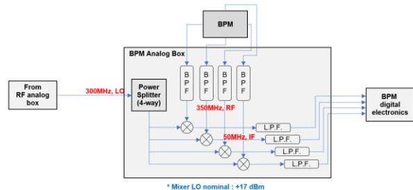
Fig. 3. Schematic diagram of the BPM analog box
