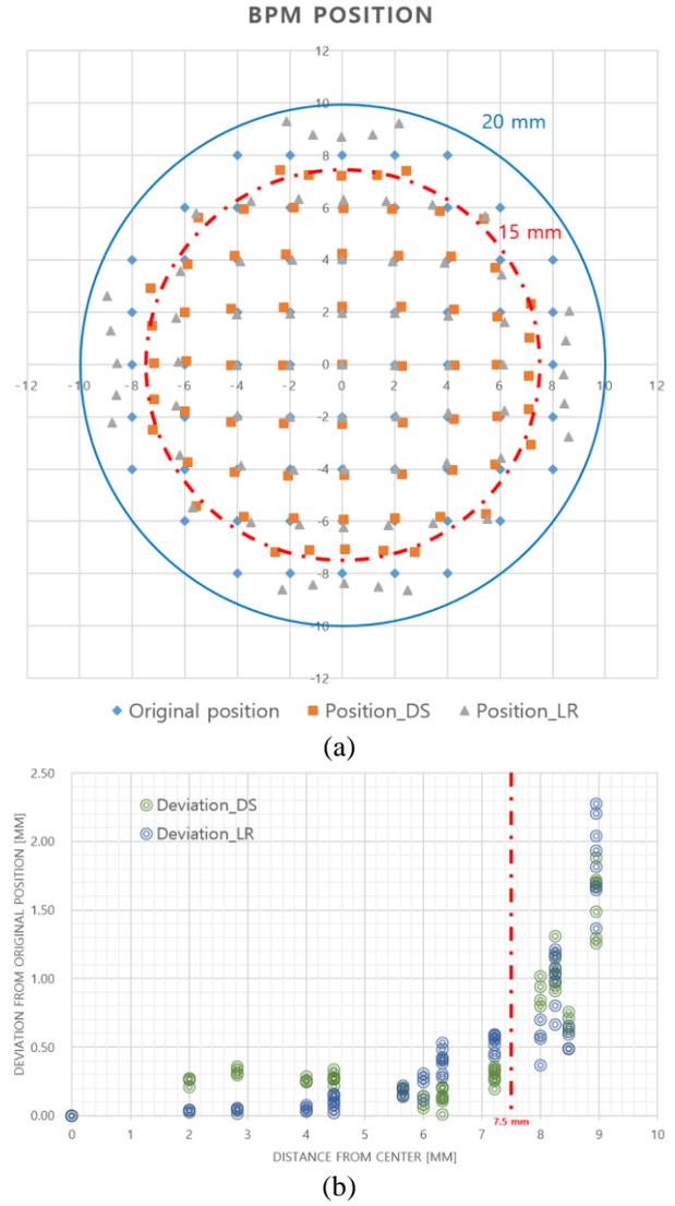
Fig. 4. Beam position difference between the original position and the measured position: (a) the position distribution on the transverse plane, (b) the position deviation vs. the distance from center.
