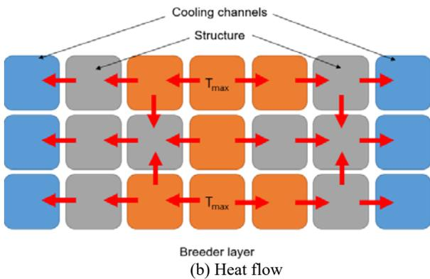
Figure 3. Heat transfer mechanism with grooved wall
