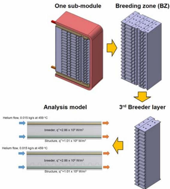
Figure 4. Geometry of analysis model
