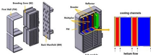
Figure 1. Exploded and internal view of the HCCR-TBM
