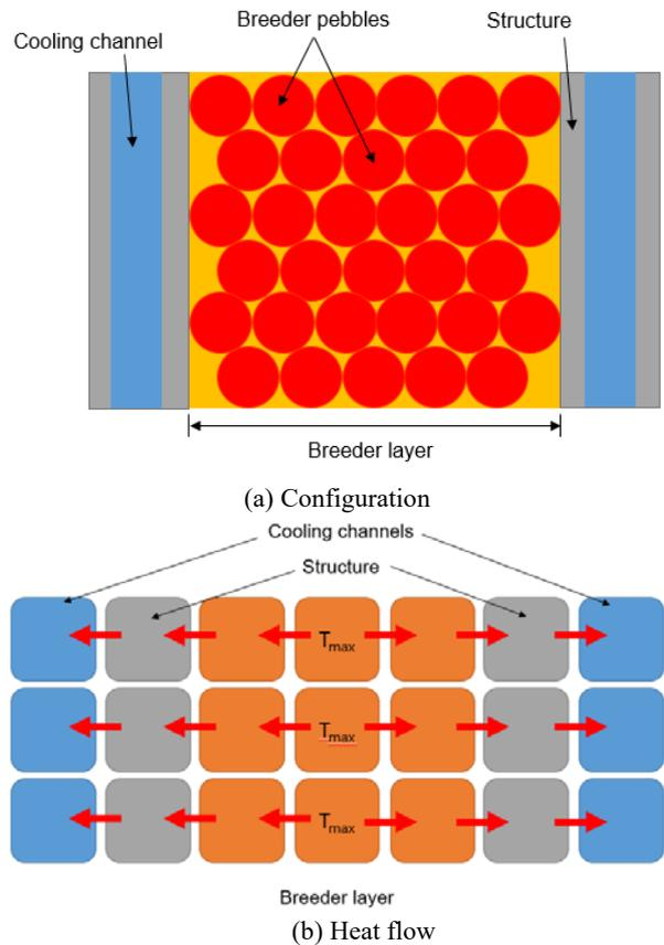
Figure 2. Original heat transfer mechanism
