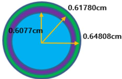
Figure A. Fuel Rod Dimensions
