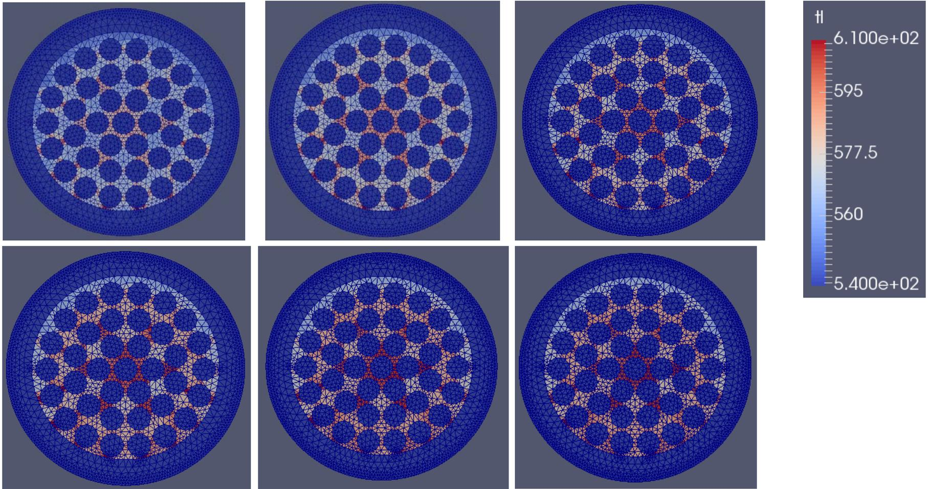
Figure 13. Coolant Temperature for Cross Section 7~12
