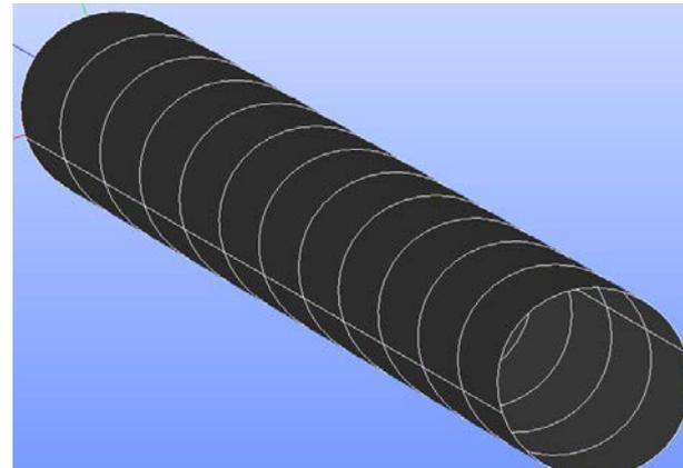
Figure E. Gap and Calandria Tube Interface(solidf4)
