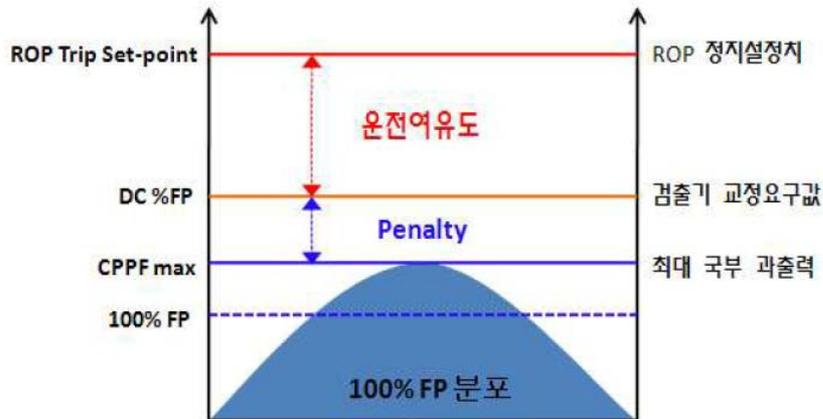
Fig. 1 ROP Trip Set Point and Operational Margin in PHWR
