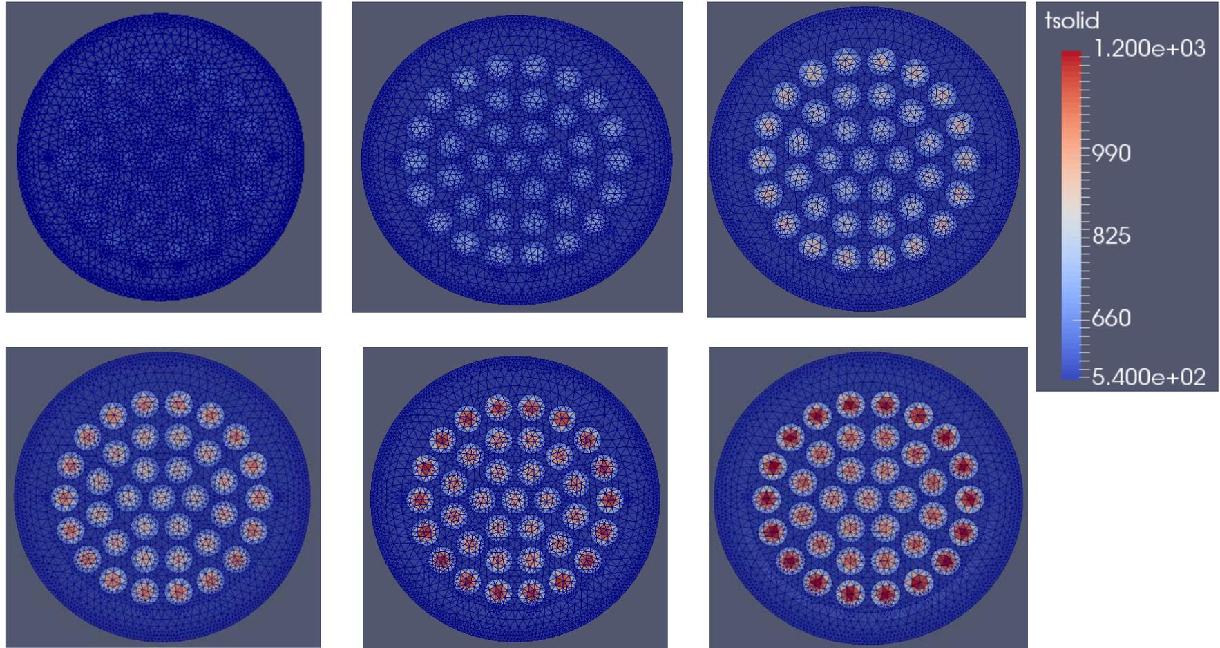
Figure 10. Fuel Temperature for Cross Section 1~6
