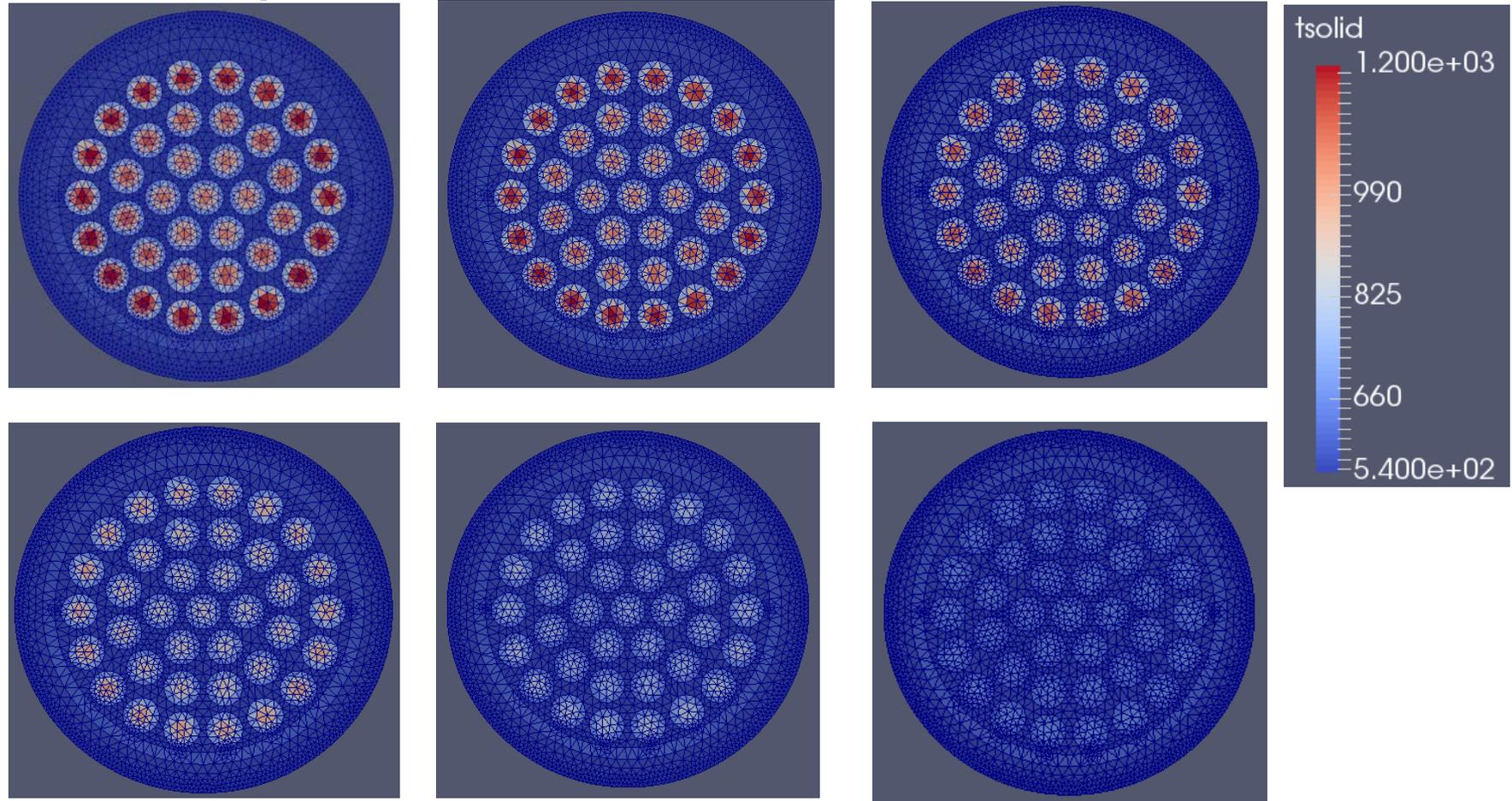
Figure 11. Fuel Temperature for Cross Section 7~12
