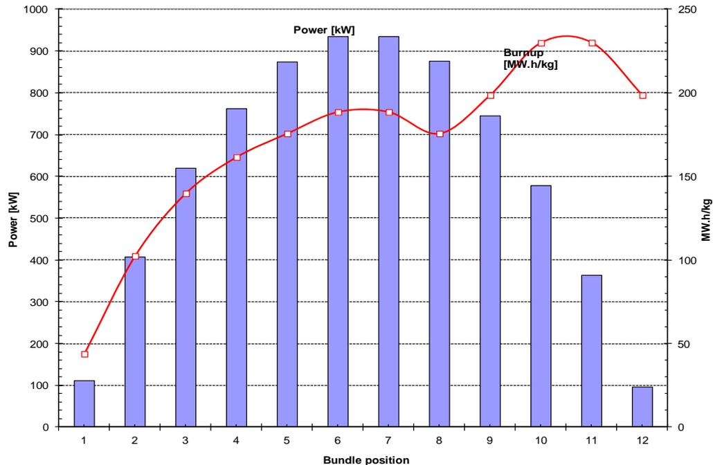
Figure 7. Axial Power and Burnup Profiles
