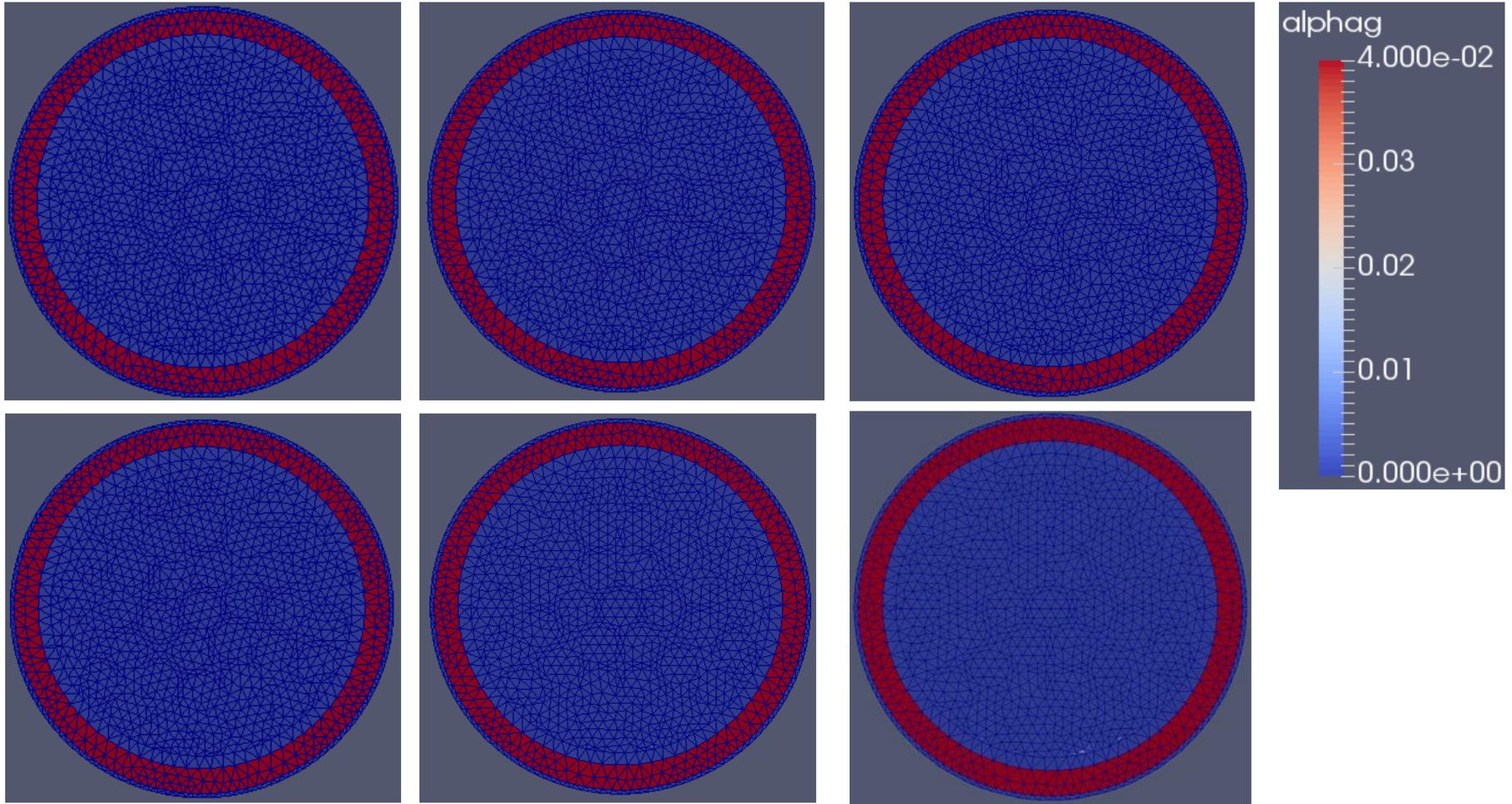
Figure 14. Coolant Void Fraction for Cross Section 1~6
