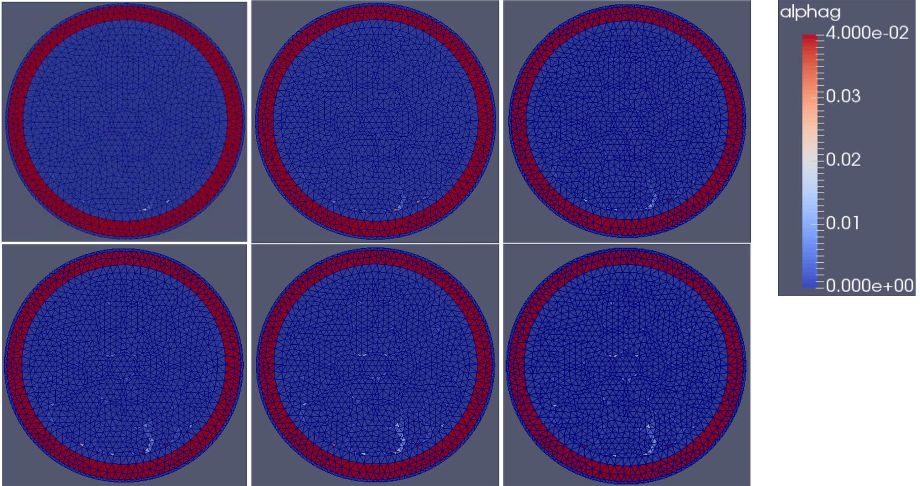
Figure 15. Coolant Void Fraction for Cross Section 7~12
