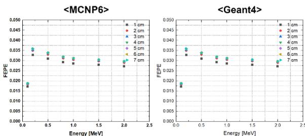
Fig. 4. Detection efficiency of GAGG(Ce) according to thickness.
