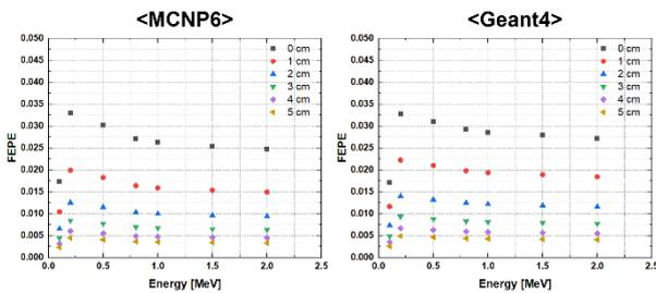
Fig. 3. Detection efficiency of GAGG(Ce) according to SDD.
