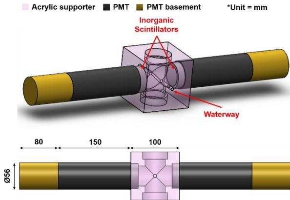
Fig. 1. Conceptually designed detection system.
