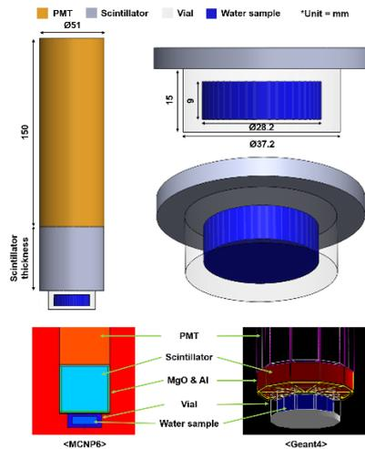
Fig. 2. Dimensions and modeling in simulations.
