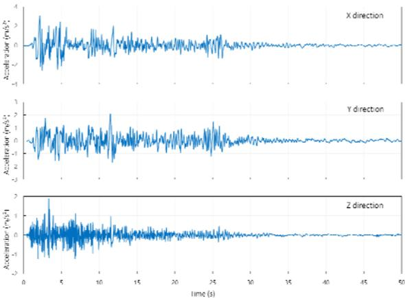
Fig. 2. Three-directional input ground motion
