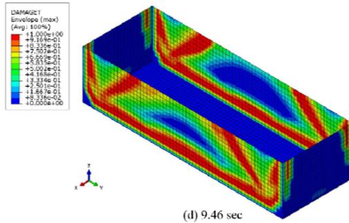
Fig. 4. Tensile damage variable  $d_t$  (continued)
