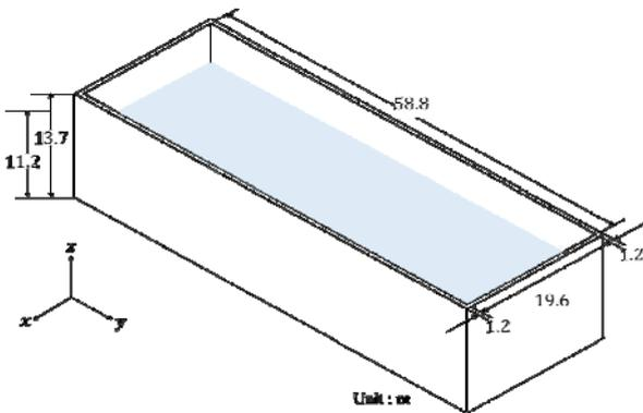
Fig. 1. Rectangular liquid storage tank
