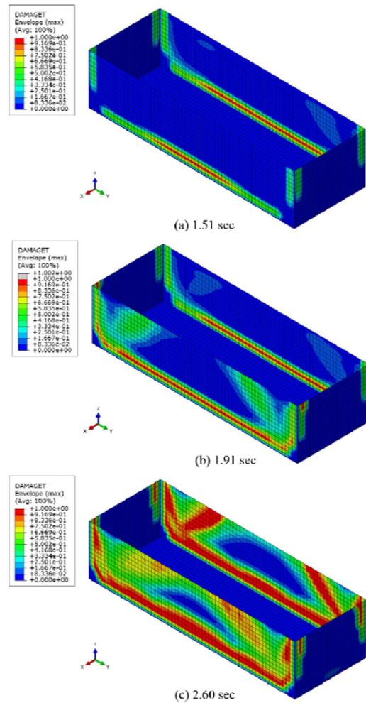
Fig. 4. Tensile damage variable  $d_t$
