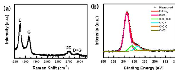
Figure 4. (a) Raman spectrum and (b) C1s XPS spectra of the GQDs.
