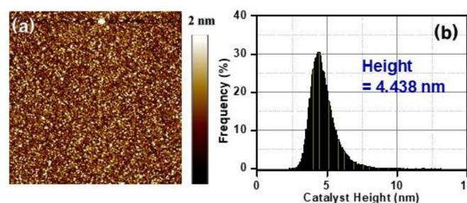
Figure 2. (a) AFM image and (b) height distribution of the fabricated Fe nanoparticles on Si substrates after annealing, respectively.
