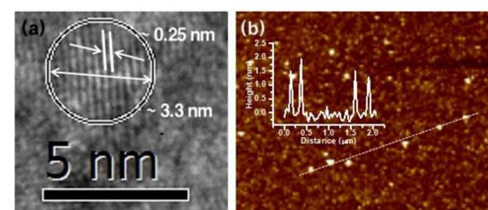
Figure 3. (a) High-resolution TEM image and (b) AFM data of the synthesized GQDs by our ion-beam assisted CVD.
