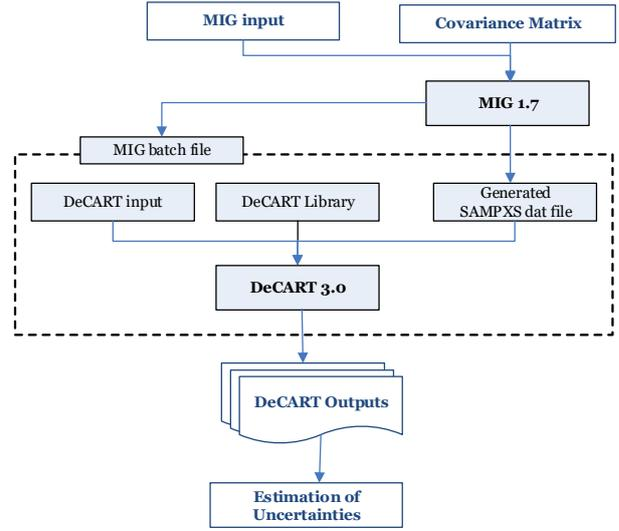
Fig. 1. Flowchart of DeCART/MIG uncertainty quantification analysis code system.
