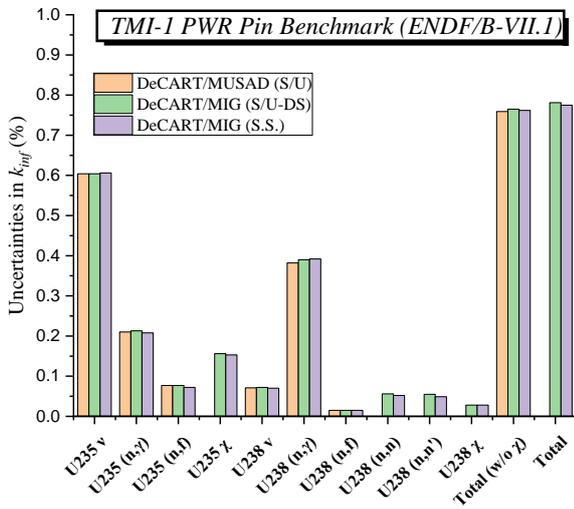
Fig. 2. Comparison between the uncertainties in  $k_{inf}$  by the S.S. and S/U method for UAM TMI-1 HFP pin problem
