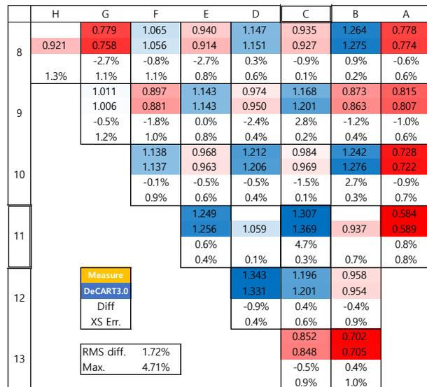
Fig. 3. Uncertainties of assembly-wise power distribution due to  $^{235}\text{U}$  and  $^{238}\text{U}$  cross section uncertainties
