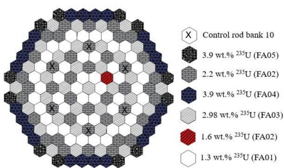
Fig. Radial layout of Kalinin-3 NPP
