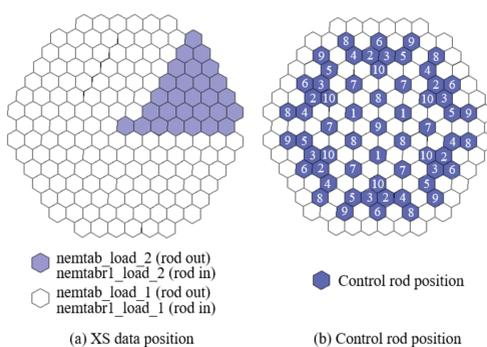
Fig. Cross-section data position with control rod bank
