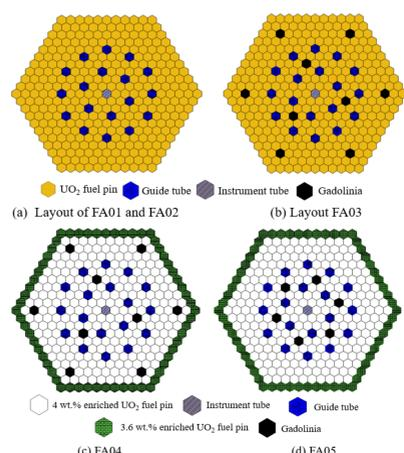
Fig. Radial layout of Kalinin-3 FAs
