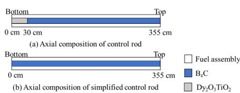
Fig. Axial composition of control rod
