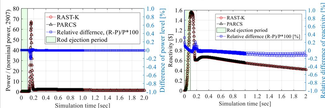
Fig. Core power of during rod bank ejection
