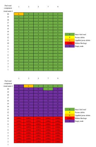
Figure 2 Core node map at the time when first core degradation occurs (upper) and at time when all the core became molten(lower)
