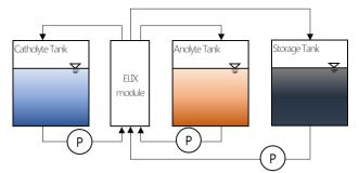
Fig. 3. Conceptional drawing of boron removal system using ELIX.
