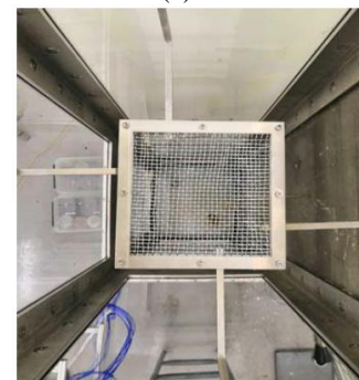
Fig. 3: (a) Mesh grid specification (b) mounting of grid in MATE tank
