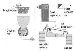
Fig. 5. Process of cable insulation separation system [4]
