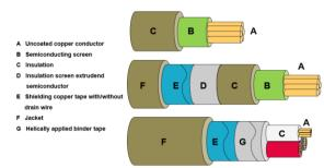
Fig. 1. Configurations of cable designs used in NPPs
