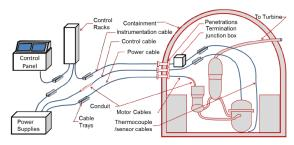
Fig. 3. Typical layout of cable system [2]
