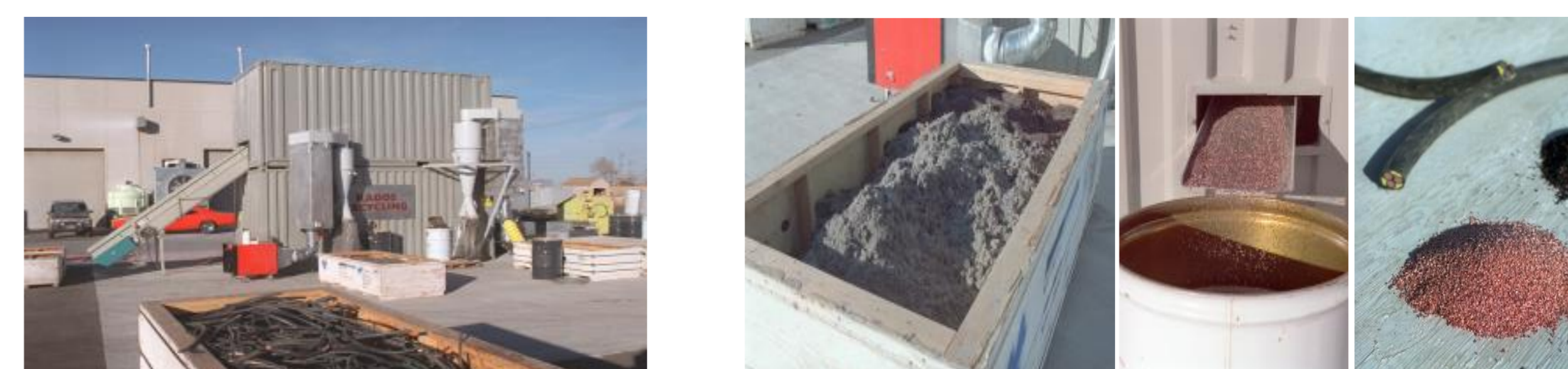
Fig. 4. Copper cable recycling system (NUKEM) and Final product using recycling cable system (dust, insulation and copper)
