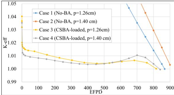
Fig. 4. The effective multiplication factor behavior of the ATOM cores
