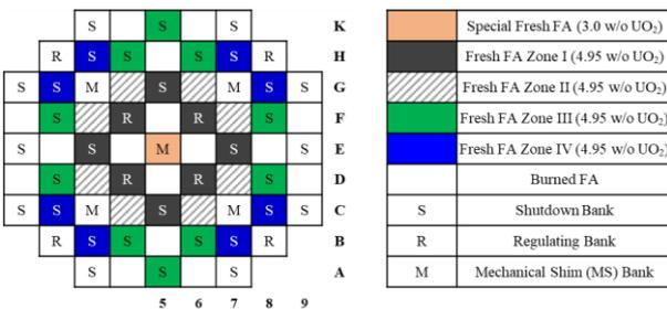
Fig. 2. Radial zone-wise fuel loading and CR pattern.
