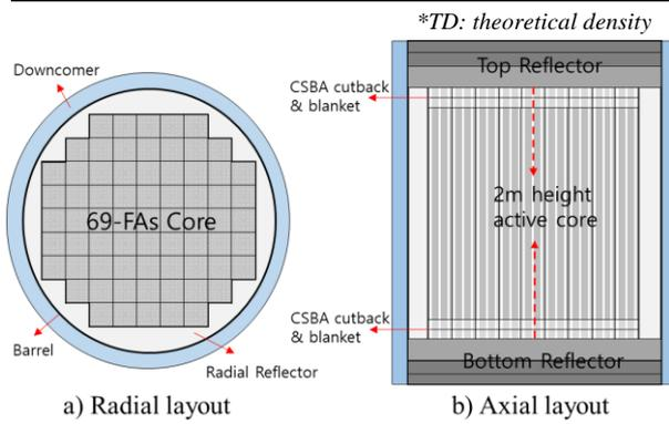
Fig. 1. The axial and radial layouts of the ATOM core
