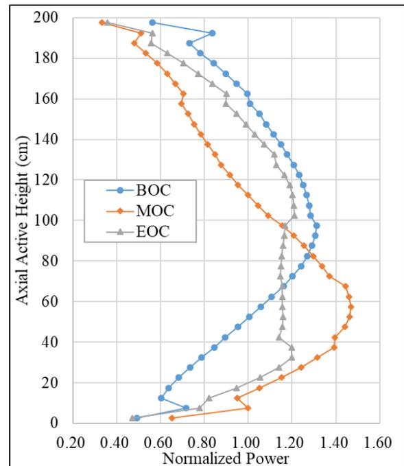
Fig. 6. Axial power distribution of the ATOM core
