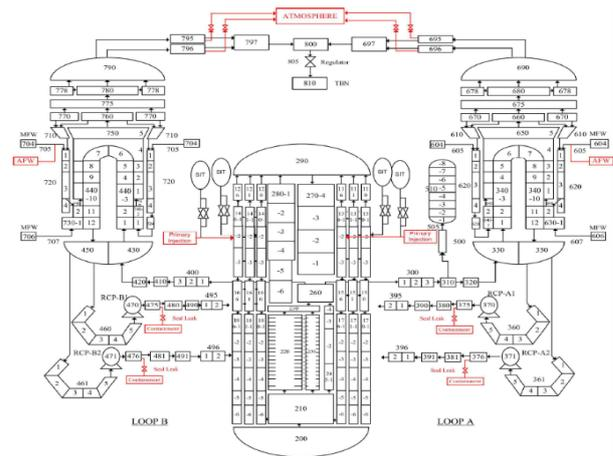
Fig. 3. APR1400 System Nodalization
