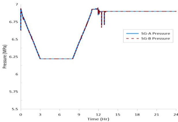
Fig. 10. Steam Generators Pressure
