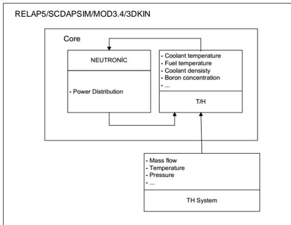
Fig. 2. Data Exchange in Coupling Neutronics and Thermal Hydraulics Modules
