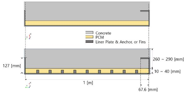
Fig. 4. Geometry scene of the non-finned case (upper) and finned case (lower) (The geometry is 90° rotated in counter-clockwise direction)
