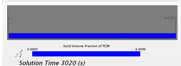
Fig. 10. Solid Volume Variation (Thickness: 30mm, Non-finned)
