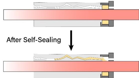
Fig. 2. Example of the self-sealing mechanism
