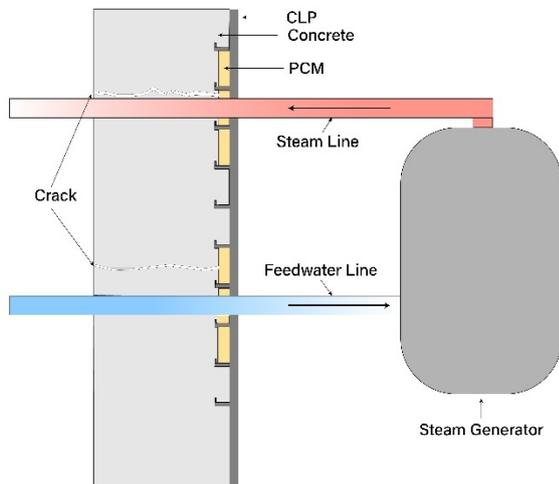
Fig. 1. Diagram of the PCM placed containment
