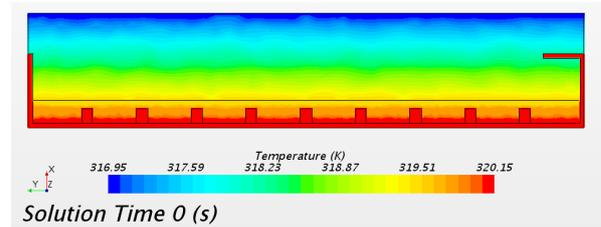
Fig. 6. Initial Temperature Distribution
