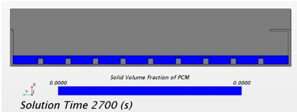
Fig. 11. Solid Volume Variation (Thickness: 30mm, Finned)
