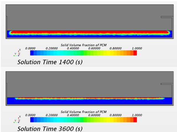
Fig. 12. Solid Volume Variation (Thickness: 40mm, Non-finned)
