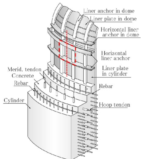
Fig. 3. Analysis object set-up
