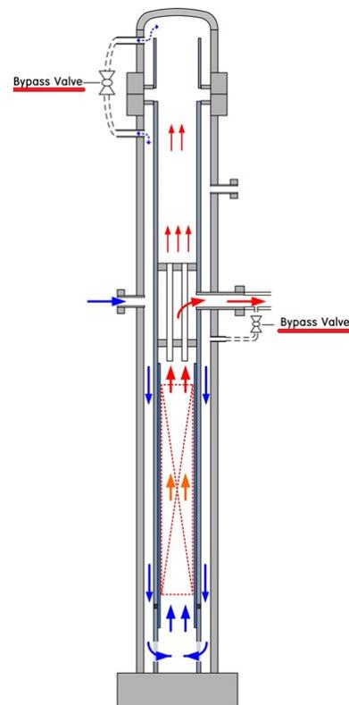
Fig. 4. Schematic diagram of RPV and by-pass valves of ATLAS
