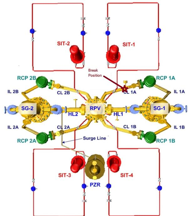
Fig. 1. Top view of ATLAS and position of break system
