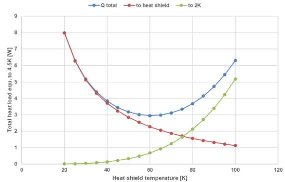
Fig. 3. Radiation heat load depending on the heat shield temperature, which is normalized to 4.5K.
