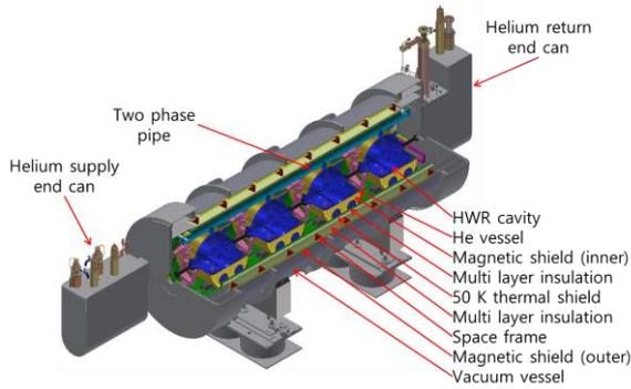
Fig. 2. Cryomodule including 4 HWR cavities for 200-MeV energy upgrade of KOMAC 100-MeV linac.
