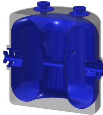
Fig. 1. HWR cavity designed for 200-MeV energy upgrade of KOMAC 100-MeV linac.
