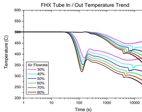
Fig. 6 FHX Tube Temperature Trend
