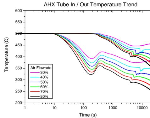
Fig. 5 AHX Tube Temperature Trend
